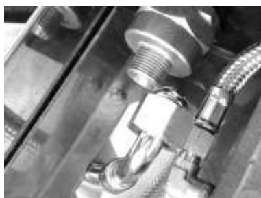
Connecting the metal hose
